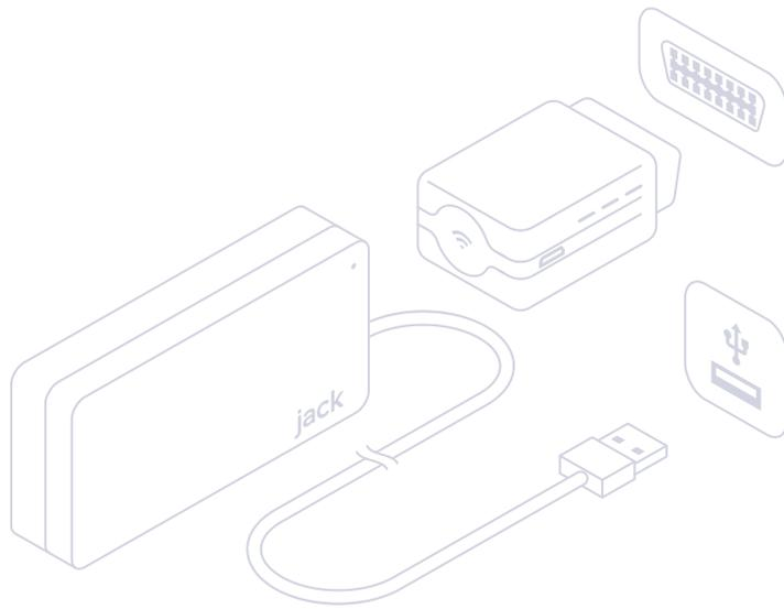
Connect the Gateway to the USB port of your vehicle or connect the dongle to the OBD port.
